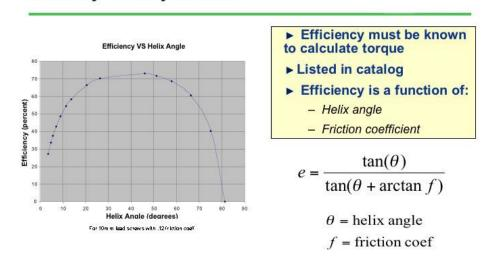
Definition: Efficiency is the ratio of work in to work out.
