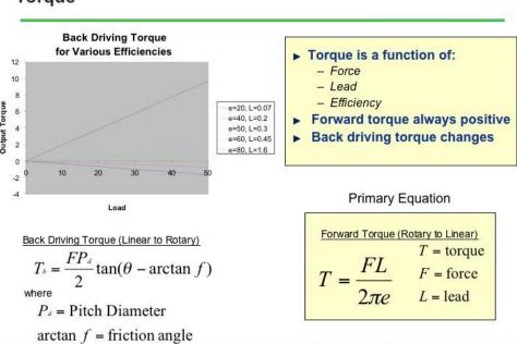
Whether metric or inch, forward torque is always positive, while back driving torque changes. The calculations would be the same when determining torque for a system in English units.
