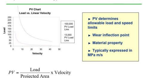
PV is usually expressed in Mpa m/s. It can indicate the wear inflection point of a chosen lead screw.
