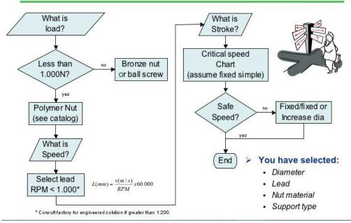
Choosing metric components for an application, for example a lead screw, is no different than choosing an English components. As seen in the flow chart, the primary factors to know are load, speed and stroke. This information will help determine the metric lead screw diameter, lead, nut material and any support.
