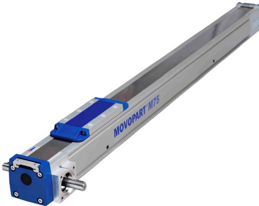
M75 Belt Image: Thomson's linear rodless actuator slides provide guided linear motion through a belt drive and saddle that rides along the top of the actuator to carry the load.
