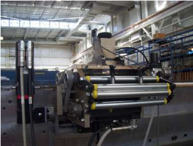
Fig 2. Dynamic Zig Zag Roll Feeder from Minster Machine with Thomson SuperSlide 2RB continuously supported systems with linear rails, integral ball screw assemblies and T-slot cartridges.
