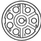
Top view build-in plug power
