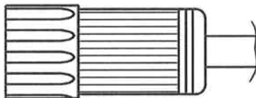
Shield connected to metallic cover
