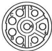
Top view build-in plug power
