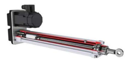
The design of a precision linear actuator is quite basic. An electric motor – through a belt gear, a worm gear, a planetary gear or via a coupling directly – rotates a ball screw which translates the torque into axial force through the extension tube.
