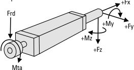
Make sure to install the actuator so that the extension tube never runs in to the mechanical end stops. The distance between the mechanical end stops (Send) are the ordering stroke (Smax) plus  $2.5 \pm 0.5$  mm of extra travel in both ends (Safe).
