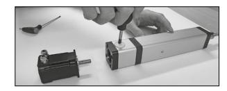
2. Press the motor shaft on to the coupling inside of the flange.
