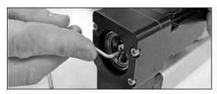
4. Bolt the motor to the flange using four screws. Tighten the screws according to table T6.3.1.
