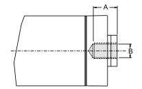
The extension tube can handle some side load (see table T6.1.1 for load and load torque data for each model) but in order to improve overall performance and life it is good practice to follow the below points even if the side loads do not exceed the maximum permitted levels.
