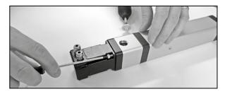
4. Use a hexagon key to tighten the coupling around the motor shaft. Correct tightening torque for PC25 models = 0.85 Nm and for PC32 and PC40 = 2.0 Nm.
