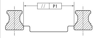
Square rails are required to have extremely parallel surfaces to prevent binding and excessive wear. They tend to take on the shape of the mounting surface so strict adherence to the parallelism specifications is necessary.
